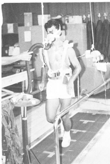
Fig 1. Application of the douglas bag method for measuring aerobic energy output dur treadmill running for the added weight condition.
