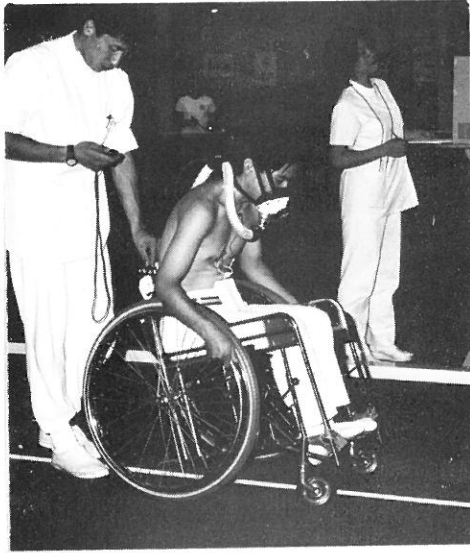
Fig 1. Application of Oxygen consumption meter for measuring aerobic energy output during wheelchair exercise.
