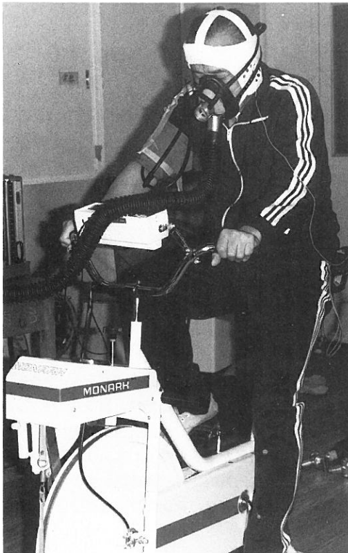
Fig.1 Application of the Douglas bag method for measuring oxygen uptake during exercise on bicycle ergometer.
