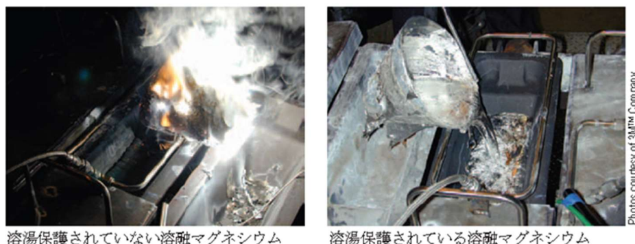
Fig. 1-17 Surface of molten magnesium protected by SF 6 gas 1-29) .
