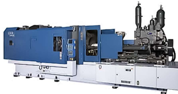
(b) Magnesium injection molding machine mechanism
